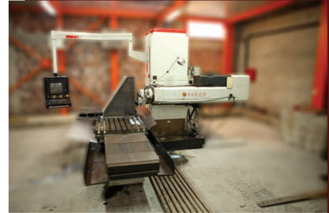
1.CNC glodalica HURON Maksimalna dimenzija obrade 2000x1200x980 mm CNC milling machine HURON (max. Size 1200 x 980 x 2000 mm)
