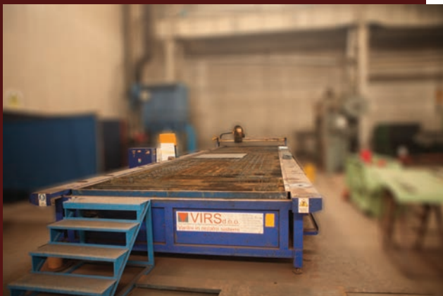
6.CNC plazma i plinsko sječenje limova Maksimalna dimenzija table 100x2000x12000 mm CNC plasma and gas cutting mashine (table to 100x2000x12000 mm)
